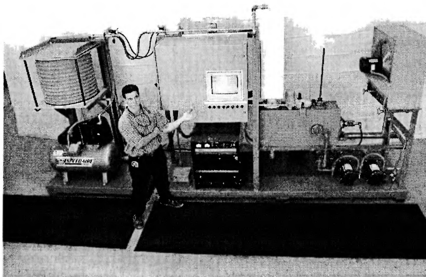
Figure 7.10. [8] A picture of a PlasmaArcFlow TM Reactor with 75 kW DC power unit which produces about 1,000 cf of magnegas per hour possessing about 870 BTU/cf plus about 500,000 BTU of heat per hour.
